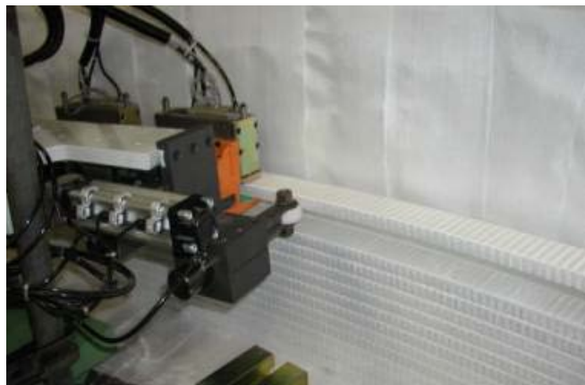
Bend conductor pressed against cylinder
