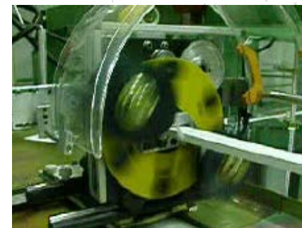
Taping insulation on conductor
